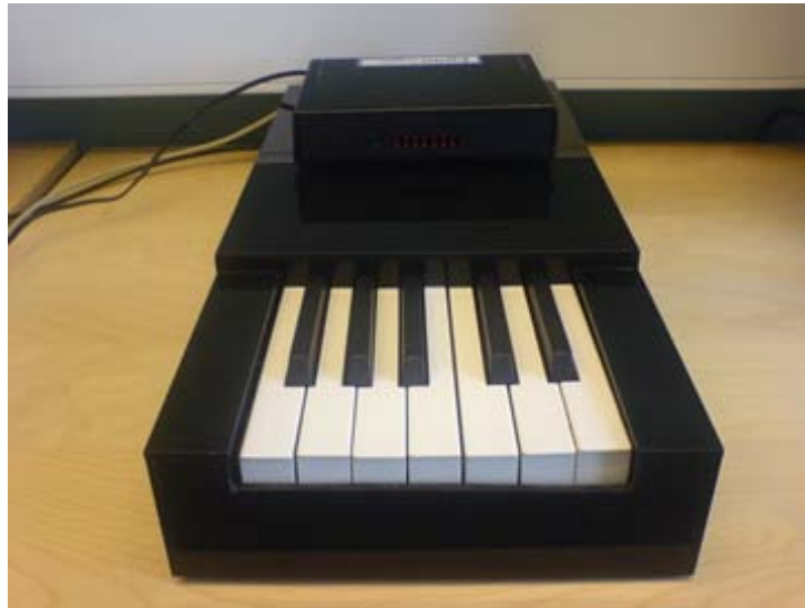
Figure 3.1: MR-compatible fiber-optic piano keyboard (LUMItouch, Inc.)
